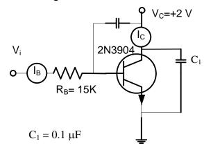
across the collector prevents oscillation that can be caused by the long leads going to the meter. The current gain,  $h_{fe}$ , depends on  $I_c$ . Specific examples can be seen in the specification sheets in the textbook.
