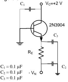
until  $V_{be}$  has the value needed to permit the resistor current to flow into the emitter. The current is determined by the voltage across R.
